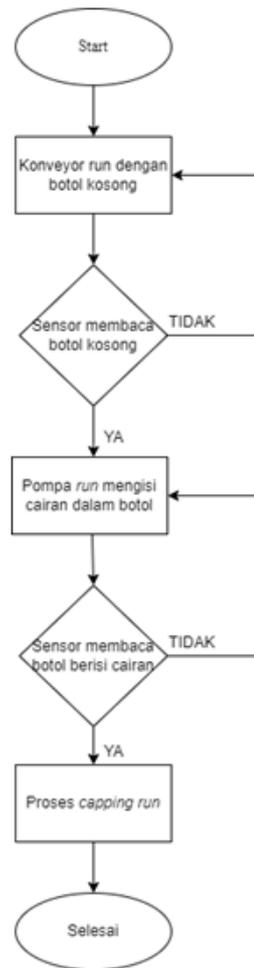
Gambar 6. Flowchart system filling capping berbasis Outseal PLC
