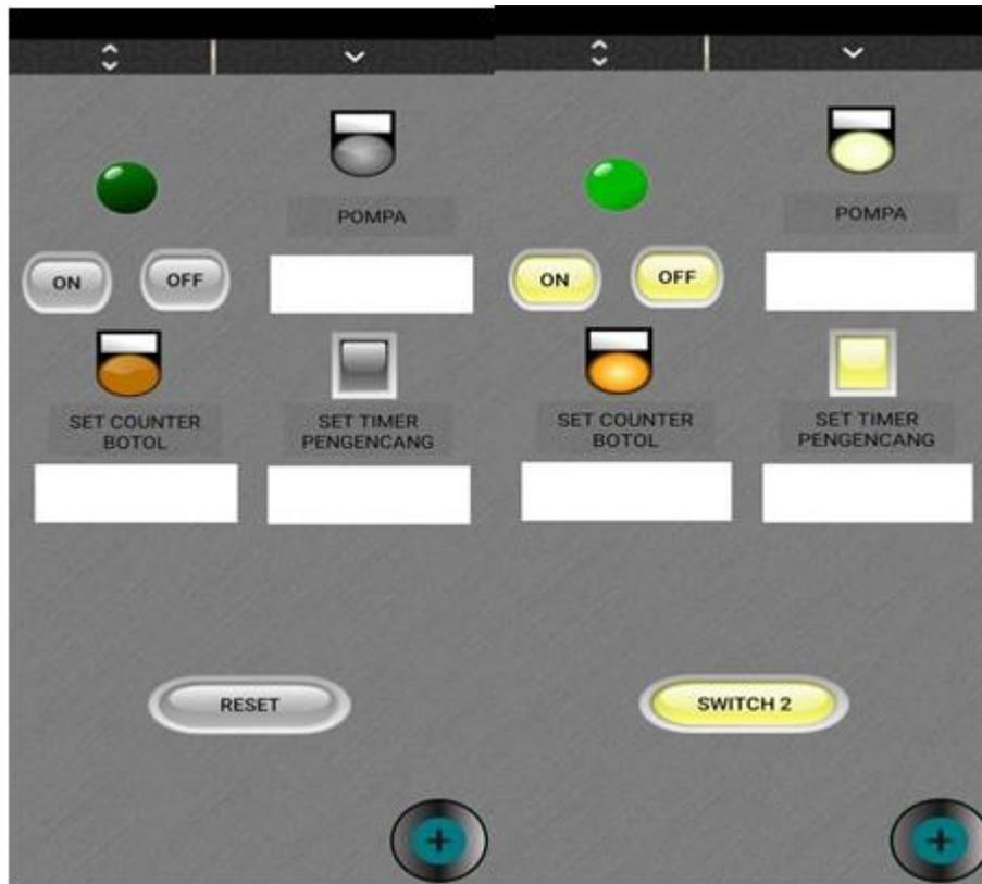
Gambar 5. Tampilan HMI Modbus system filling capping berbasis Outseal PLC
