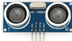
Gambar 10 Sensor ultrasonik
