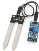
Gambar 11 Soil Moisture Sensor
